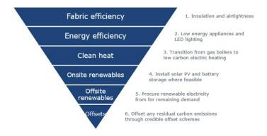
This is referred to as a 'Fabric First' approach and is accepted as best practice to decarbonise buildings. Upgrading the fabric increases energy efficiency and reduces demand for energy and carbon emissions. It also prepares the building for the transition to low carbon heat, and often reduces the cost of installation through reduced systems sizes and future electricity consumption.
